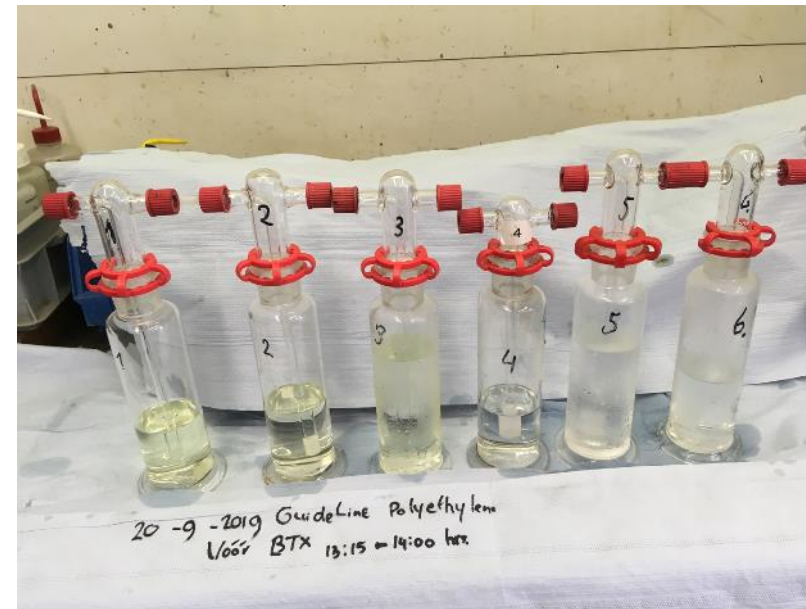
After Olga Tar removal
